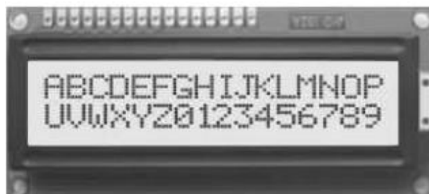
Gambar 2.5 LCD 16x2 Sumber: (Soni & Suchdeo, 2012)
