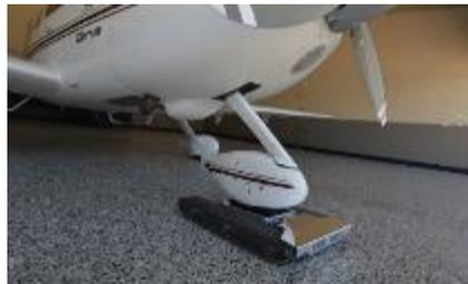
Figure 1 Towing tug remote control
