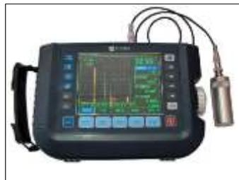
Gambar 1. Alat uji *ultrasonic Flaw Detector* TUD 310.
